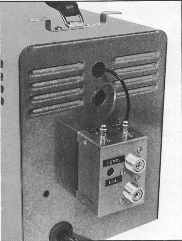
Figure 1: Rear section of WO-33A oscilloscope case with W2GQK's RF sample-box mounted and connected.
